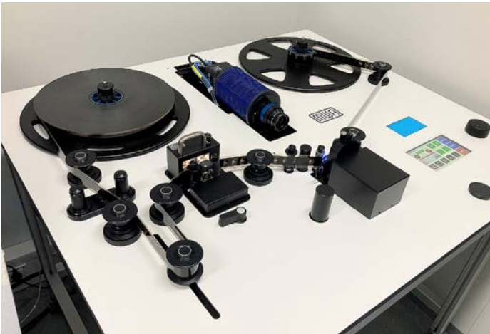
↑ Our MWA Spinner S2 multi-format film scanner, which is integrated into the ZMKK national research infrastructure.
